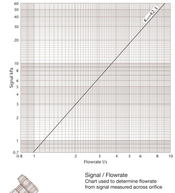
$Q = Kvs \sqrt{\Delta p}$ 36 Where Q = Flowrate I/s  $\Delta p = Signal kPa$ Kvs = Signal Co-efficient
