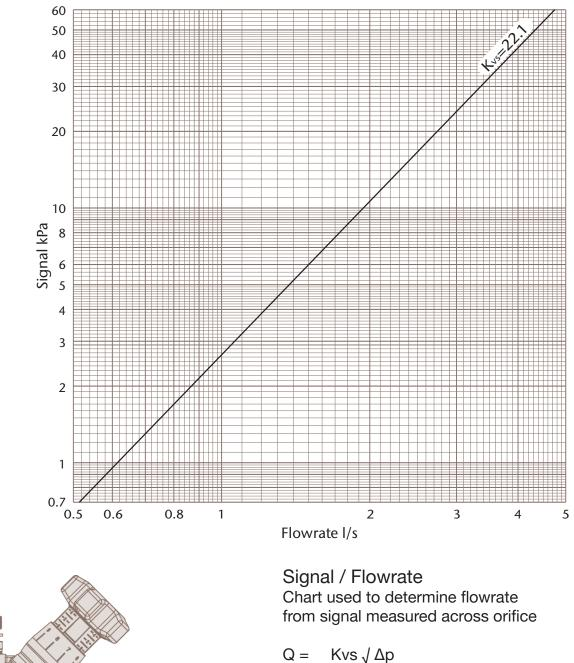
$Q = KVS \sqrt{\Delta p}$  36Where Q = Flowrate I/s  $\Delta p = Signal kPa$ Kvs = Signal Co-efficient
