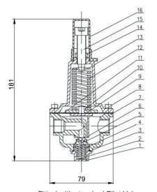
Fitted with standard Pilot Valve 0.70 to 12.00 Bar (10 to 175 PSI) Factory set to 2.5 Bar (36 PSI)
